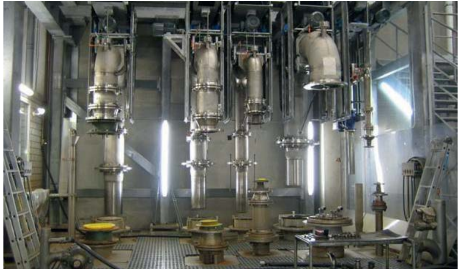
The high pressure test stand at Schroeder Valves can generate a maximum pressure of 400 bar and simulate fluctuating load conditions.
